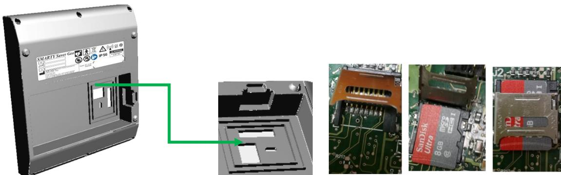
The data recorded directly on the  $\mu$ SD memory can be downloaded and displayed on a PC using the PC Saver View Express software owned by Ami Italia.
