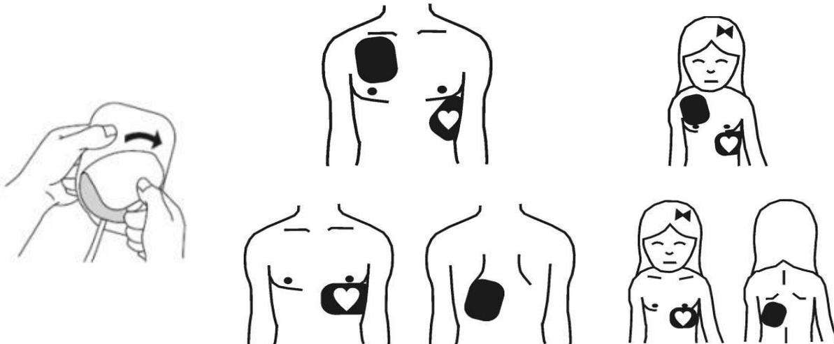
The correct placement of the pads is essential for an effective analysis of the patient's heartbeat and for the consequent delivery of the shock, if needed.
